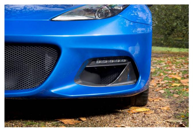
Cumulatively this all works to boost downforce to 96 kg at 190 mph, a sizable jump of 50% over the outgoing Evora Sport 410, and a massive three-times that of the Evora 400 with an improved drag coefficient. This elevates the Evora GT410 Sport to the top ranks of Lotus' most aerodynamically efficient road cars.
